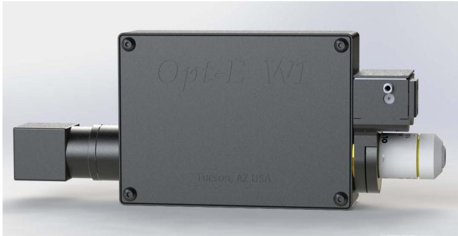
*The Opt-E W1-IM interference microscope for surface profiling is based upon the W1 reflected-light microscope body. We add to it an nPoint piezo-stage for fine focus and phase-shifting and a Nikon Mirau interference objective to produce a compact instrument for surface profilometry.*
