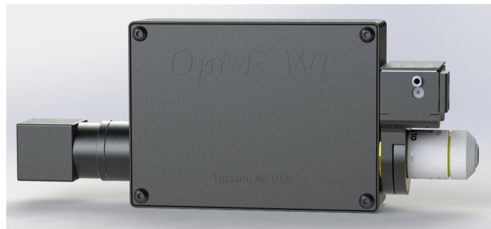
Figure 1. W1 reflected light microscope with C-mount camera on the left and PZT mount on the right. The PZT mount can be used for focusing as well as phase-shifting interferometry or coherence scanning interferometry. A standard RMS objective is attached.
