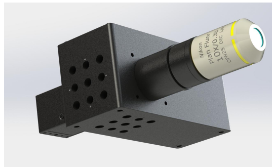
Figure 1. W2 alignment module with 100 mm focal length collimating lens and Nikon 10x objective installed. Removing the objective exposes a 12 mm diameter collimated beam with the standard 100 mm focal length collimating lens.
