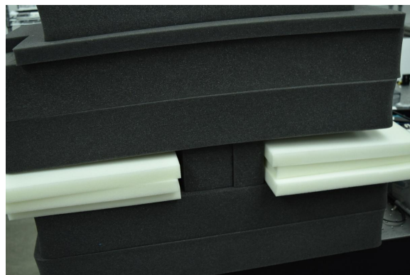
Figure 11. The W2-AM was then placed inside a stack of foam with 8" (200 mm) or more foam in each direction.
